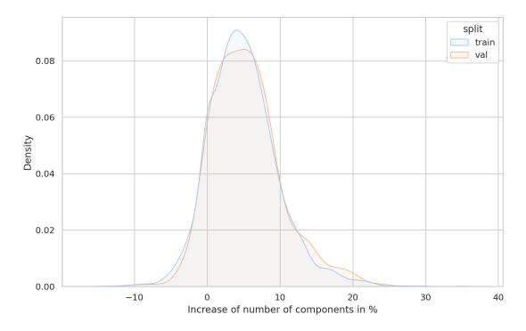
Assessment of object stability under morphological opening - erosion followed by dilation. When many components are small, the number of components decreases, which means we might have noise in our annotations (i.e 'sprinkles').
